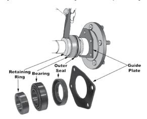
Wheel Cylinders, etc. Clean and inspect the Bearing surfaces.
