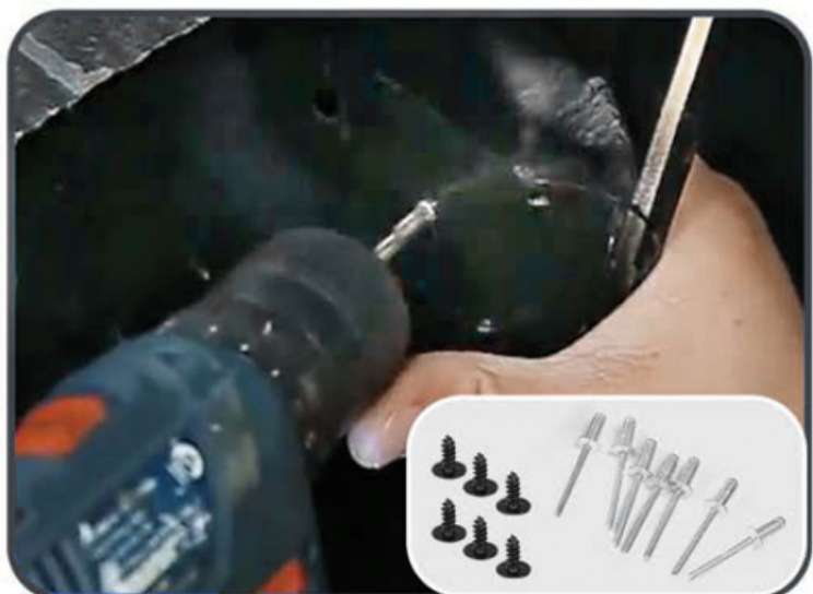
3. Fix the bracket by screws or rivets
