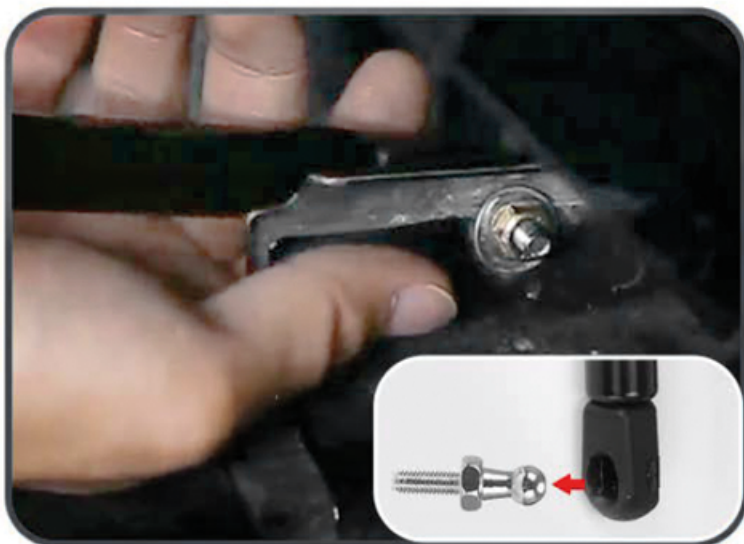
1. Fix the bottom of the hood
