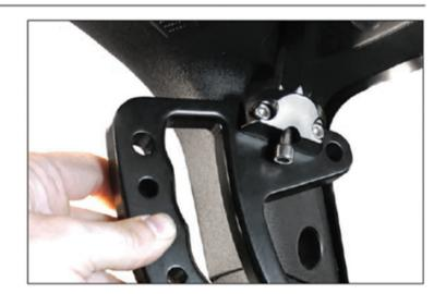
6. Now tighten bolts in a alternating pattern to avoid components from binding up. DO NOT use power tools. Tighten the two bolts snug but do not over tighten to avoid striping the threads or breaking the bolt.
