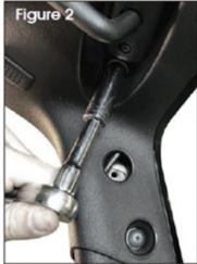
5. The handle requires some preassembly. Use the small allen head bolts to attach the mounting cup to the handle. The cup protion will be to the top of the handle.
