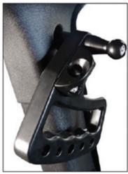
8. Now take the shorter bolt insert into the handle and then the hex spacer while rotating the handle into position. This can be a little tricky to align so take your time to avoid cross treading.
