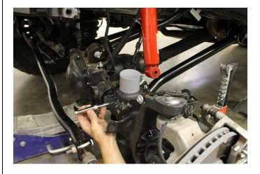
28. Remove top front coil spring isolator
