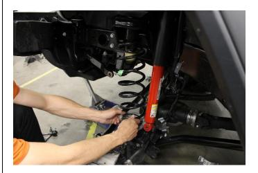
27. Install bump stop using provided hardware
