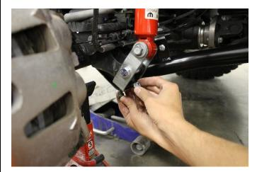
32. Install lower shock mount using factory hardware
