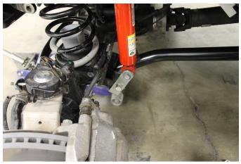
33. Install factory rear sway bar end linka. Use factory rear sway bar link in placeof the front sway bar link
