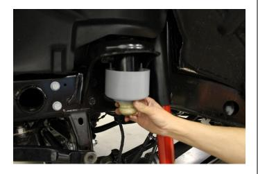
30. Install factory coil spring
