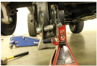
14. Install lower shock mount using factory hardware
