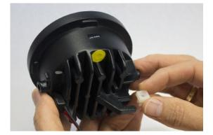
**4.** Align the back fin on the lamp with the screw hole on the plastic housing. Snap the lamp into the housing starting with the side closest to the white nut.
