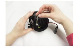
**7.** Plug in the lamp and turn on the fog lamps while holding the lamp in place. Compare the pattern of the light coming from the 2 fog lamps as the shine on the wall by covering and uncovering each lamp individually.
