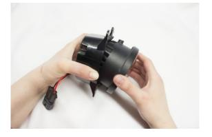
**6.** Hold the lamp assembly into the bumper. Use the 4 mounting holes to align it into position.
