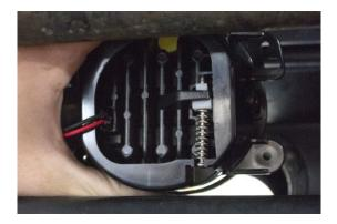
**8.** Rotate the adjustment screw (clockwise to raise, counterclockwise to lower) on the rear of the lamp to aim the light like the existing fog light.
