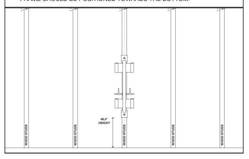
**3** POSITION/ MARK THE MOUNTING POSITION. USE THE BRACKET FOR REFERENCE AND DRILL 1/4" PILOT HOLES IN EACH STUD CENTER. PILOT HOLES SHOULD BE AT LEAST 2" INTO THE STUD. ASSEMBLE AND INSTALL THE DOOR STRAP RETAINERS BY SCREWING INTO NUT RETAINERS.
