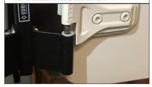
6 ADJUST THE DOOR STRAP RETAINER VIA THE ADJUSTABLE PEG FOR DOOR RETENTION. WEAVE STRAP AS SHOWN AND ELIMINATE SLACK. REPEAT FOR THE REMAINING DOOR. PROPER ADJUSTMENT PREVENTS DOOR FROM SWINGING OUTWARD.
