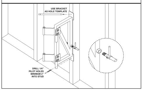
**4** DETERMINE THE PROPER LENGTH 5/16" LAG BOLTS FOR YOUR APPLICA TION. BOLTS MUST BE EMBEDDED AT LEAST 2" INTO STUD. USING 5/16" LAG BOLTS AND 5/16" FLAT WASHERS, ATTACH THE DOOR HOLDER BRACKET TO THE WALL. TIGHTEN THE UPPER DOOR SUPPORTS FULLY.
