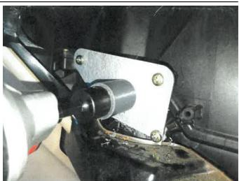
**STEP 10:** Back out the precision hole saw tool from the mounting plate. Remove the screws holding the mounting plate (Qty 3). Remove the mounting plate. Remove any plastic shavings or other debris left at the entry point into the HVAC module.
