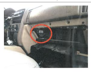
**STEP 4:** Remove the air temperature actuator from the HVAC module to access the temperature door shaft. It is not necessary to disconnect the power source from the actuator.
