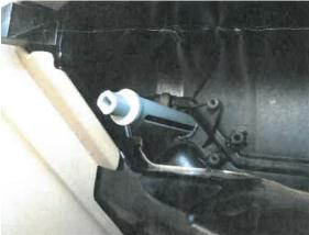
**NOTE:** To align the actuator repair sleeve with the temperature door shaft, insert the repair sleeve with the slot pointing toward the front of the vehicle at a 4 o'clock position.
