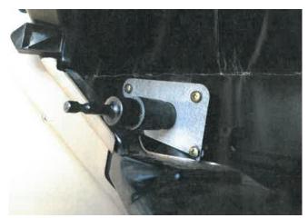
**STEP 9:** Attach a battery powered drill to the precision hole saw tool. Drill at a moderate speed until the outer sleeve of the precision hole saw tool bottoms out onto the mounting plate.
