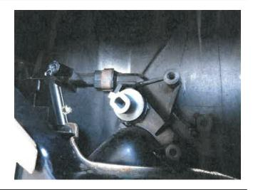
**STEP 12:** Align the air temperature actuator with the actuator repair sleeve and rotate into an engaged position.
