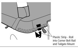
Note: The Plastic Protectors sewn into the fabric must be properly located to minimize abrasion between the Duster and the Soft Top Hardware.
