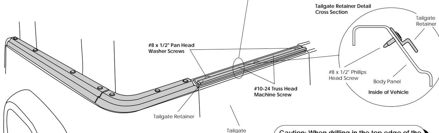
**Caution:** When drilling in the top edge of the vehicle body, check underneath for wiring. Pull the wiring out of the way before drilling.
