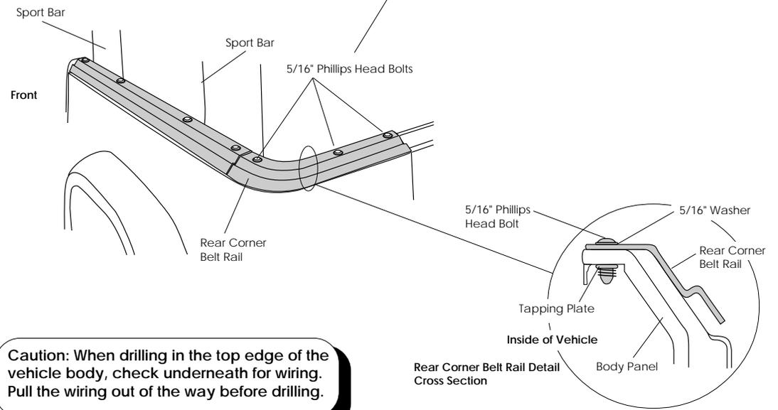
**Caution:** When drilling in the top edge of the vehicle body, check underneath for wiring. Pull the wiring out of the way before drilling.
