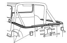
Leave packing tape on Bow Assemblies until front holes of Bow Mounts are secure
