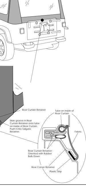
onto the tube inside the bottom of the Rear Curtain. Roll the Rear Curtain Retainer into the top of the Corner Belt Rail. Slip the plastic on the bottom of the corners under the bottom of the Corner Belt Rail. Close the rear curtain zippers.
