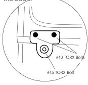
Wrangler/YJ Windshield Adjustment: If necessary, loosen the #40 TORX bolts in the windshield clamps to loosen the windshield in order to slip the bracket under the horizontal tube.
