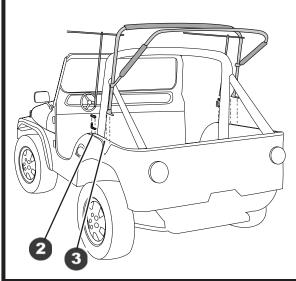
When drilling in the top CAUTION edge of the vehicle body, check underneath for
