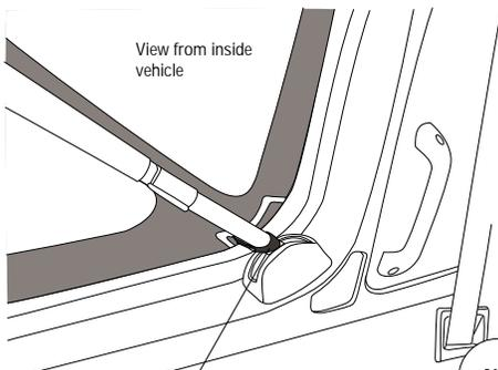
**Note:** To close Side Panel Retainer, push the retainer into the clip mounted to the body.
