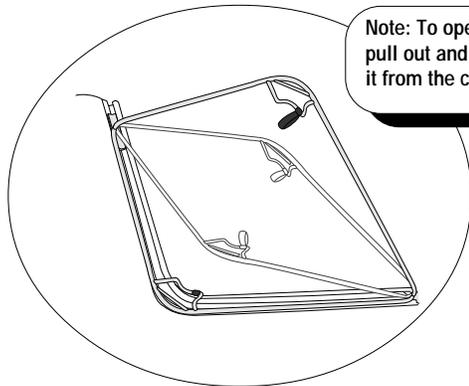
**Note:** To open Side Window Retainer, pull out and up on the retainer to release it from the clip mounted to the body.
