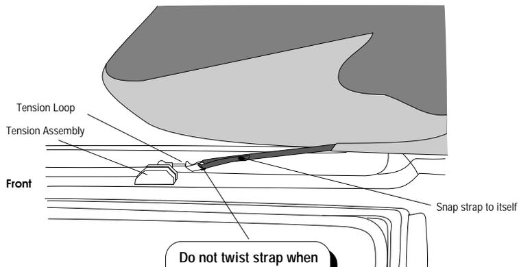
**Do not twist strap when threading through loop**
