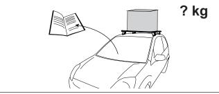
When these roof racks are to be used on a vehicle that is driven off sealed roads the maximum load rating must be divided by 1.5. Remember to subtract the weight of the roof racks to determine your maximum permissible load capacity.
