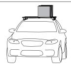
Up to, 2 bars 100kg (220lbs) load rating (Urban road) 2 bars 66kg (145lbs) load rating (Off road)
