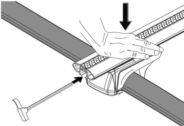
With Torque Key inserted, turn clockwise until handle straightens as below. This indicates 4-5 Nm. More pressure may be required in extreme climates.
