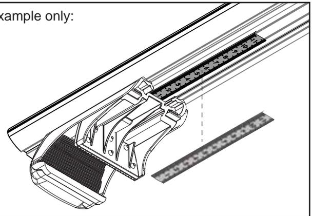
**10** Insert End Cap. Lock with Key provided and remove the Key.
