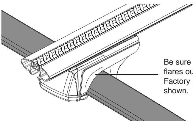
Be sure the Gasket flares out over the Factory Rail as shown.
