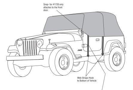
For ease of installation: Firmly hold web and buckle up with one hand while engaging the buckle lever down with the other
