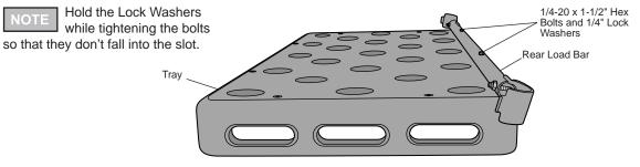
DO NOT overtighten the bolts that attach the Pillars **CAUTION** to the Tray. This may strip the aluminum inserts in the Trav.
