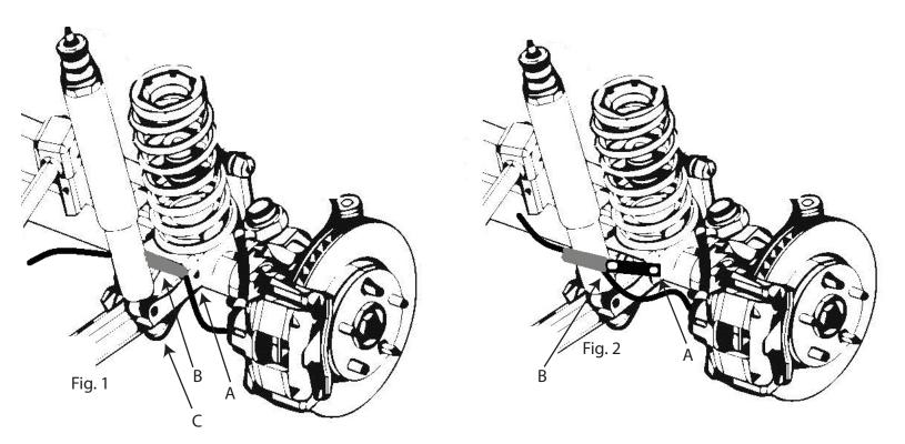
Step 1A. Remove the factory bolt holding the brake line bracket to the spring mount . (See fig. 1A)
