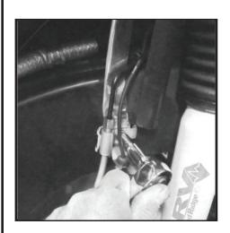
91 - (Note: 3.6L Only) Tube can be adjusted if additional clearance to heat shield is needed. Grab tube and bend as needed. Make sure lower section of air tube still clears power steering pump and hose (arrows). 92 - Tighten all 3" hose clamps.
