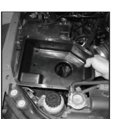
57 - If air box does not fit within 1/8" of rubber retainer grommets the top of the silicone air tube will need to be trimmed. Remove air box and elbow. If air box fits correctly proceed to step (59).
