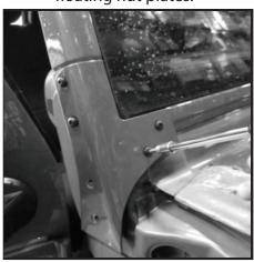
75 - If used, windshield light mounting brackets should be installed at this time.
