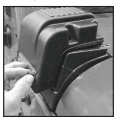
113 - Press top of intake down onto snorkel body. Intake will fit over top front of main body intake and pop over the rear of intake as shown.
