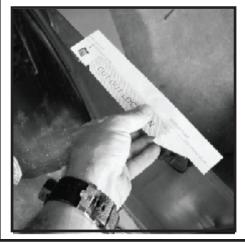
27- Align fold and guide cut outs on fender. Secure with tape. Mark holes on fender as shown. If template does not fit correctly refer to page 22 for instructions.
