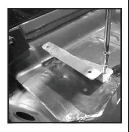
77 - Dry fit main body, elbow and air tube before applying sealent. If all parts line up apply a thin bead of sealant around the lower section of the snorkel main body. Spread sealant evenly around the outside of the outlet. A thin layer will insure a tight seal.
