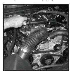
97- For 2012 - Present 3.6L models rotate 3" intake tube back into place and loosely attach to upper air box. Connect crank case hose and wire harness.
