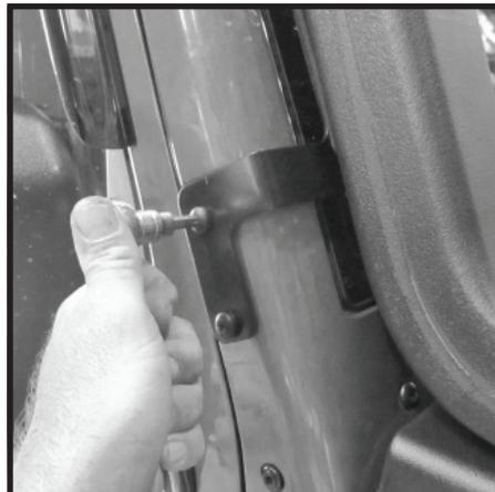
**9** - Tighten mounting bracket to high intake M6 bolts. Turn on windshield wipers to check for clearance. Adjust as needed. NOTE: vehicle must be equipped with OE correct 16" wiper blades.
