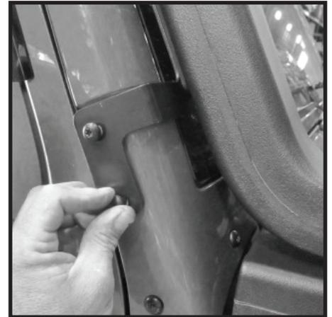
**7** - Insert (4) M6 caps head bolts and washers through intake to snorkel main body. Tighten bolts. DO NOT OVER TIGHTEN. Tighten enough to insure tight fit of gasket to snorkel main body.
