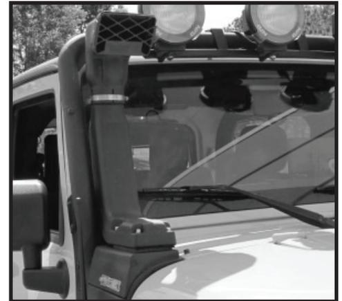
**PLEASE NOTE:** Modular high mount XHD intake has been designed for use with Rugged Ridge accessories. If vehicle is equipped with another manufactures accessories modification to accessories may be required. It is recommended that no modifications are made to the snorkel or snorkel intake system. Modifications to intake may result in reduction of vehicle performance.
