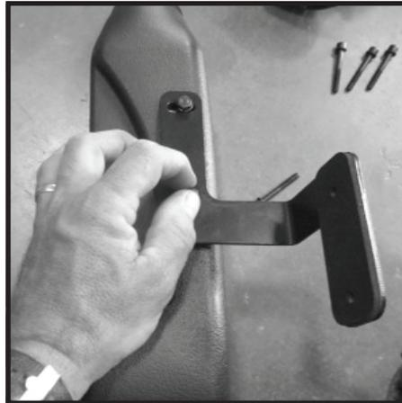
**6** - mount bracket and intake to windshield bracket using T-40 torx bolts removed in step (4). Secure bolts but do not tighten.
