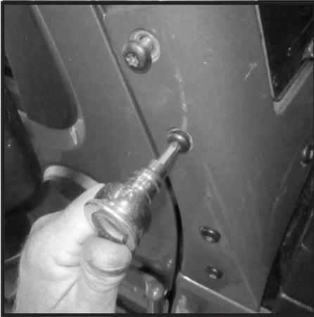
**5** - Install mounting bracket the back of high mount intake using (2) M6 hex head bolts and washers. secure bolts but do not tighten at this time.
