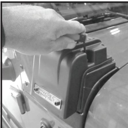
**2** - Remove lower (2) M6 side mount caps head bolts. Remove logo plate but do not discard. It will be reused. Do Not discard hardware. It will be reused if low mount intake is to be installed at a later date.
