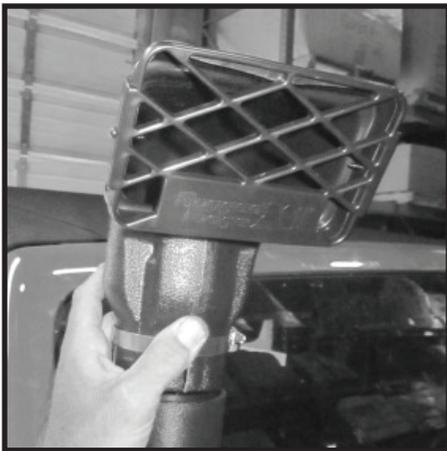
**11** - Position ram intake as low as possible onto high intake. Slide 3" clamp as far down on ram intake as shown. Check orientation of ram and tighten clamp.
