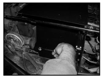
3. Install Edge Trim onto heat shield and trim to length. Install Rubber Mount to Heat Shield using supplied hardware
