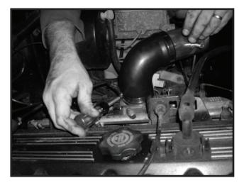
5. Align Intake Pipe bracket with Rubber Isolator Mount on the Heat Shield and fasten with washer and nut. Install Air Filter to the end of the Intake Pipe using a supplied Hose Clamp. Note: This filter is polyester synthetic and never needs to be oiled. It can be cleaned with warm water and mild detergent dish soap.
