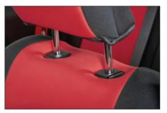
Finally, Install headrest covers and reinstall headrests.
