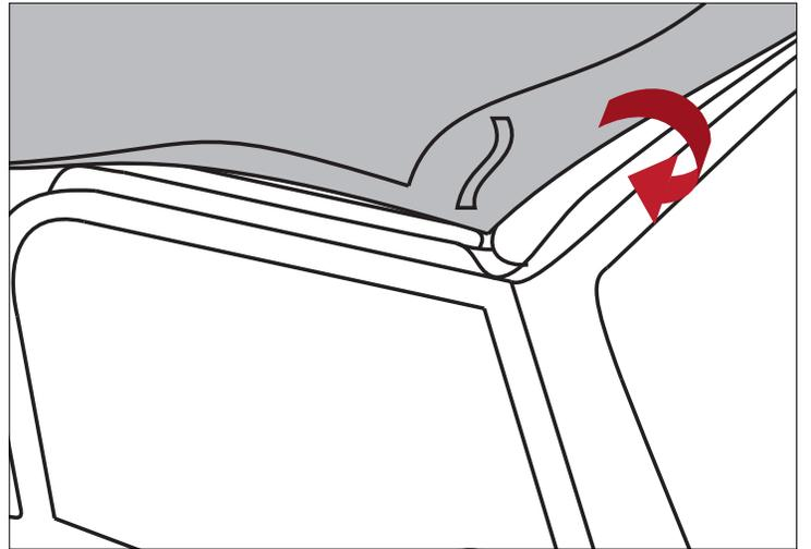
7. Insert plastic into top of door surround channels above either door opening. This will center top at front. Check that front plastic is near front of windshield channel.
