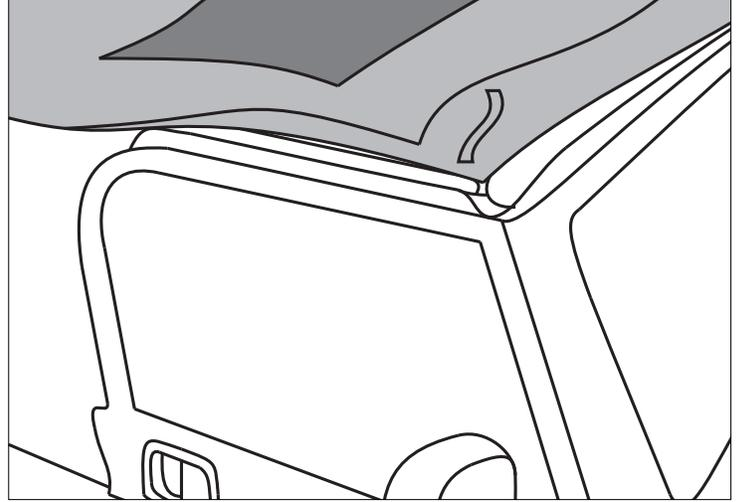
6. Insert front plastic into groove of Windshield Channel. Ends will match nearly to each end of Windshield Channel. From front of vehicle, ensure that top is even from side to side. Check door surround sides and push top toward rear to ensure fabric is seated tightly around front corners.
