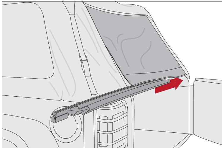
13. On top of rear part of roll bar, pull side to side adjustment straps snug, do not over tighten. Pull three rear window straps snug.
