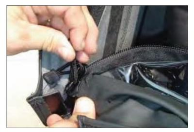
19. Remove fabric upper doors from vehicle. Using razor blade, cut stitching on old door covers and remove from frame.
