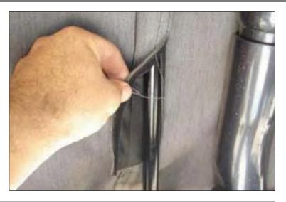
4. Release soft top snaps from rear bow and allow bow to drop on tailgate.
