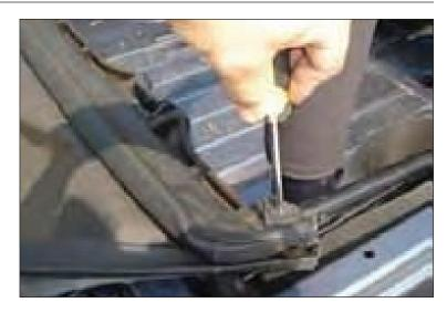
6. Flip top fabric into rear of vehicle so fabric lays bottom side up. Remove screws that fasten soft top fabric to windshield header and set aside for later use. Remove soft top fabric.
