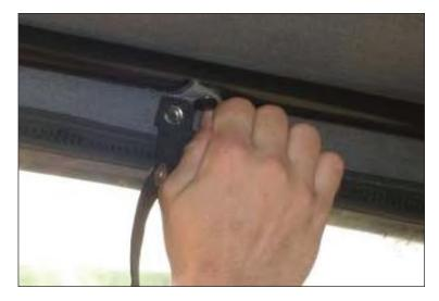
3. Pull down on spreader bars and push rear support bow forward.
