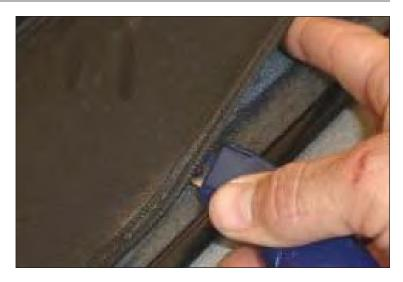
18. Separate hook and loop fasteners on new door skins. Lay door skin on flat surface with outside facing down. Start by working lower rear corner of door frame into pocket in lower rear corner of door skin. Continue working door skin around frame and fasten hook and loop strips as you go.
