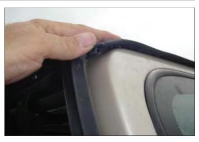
8. Push front support bow fully forward. Bow must slip into notch in belt rail. Pull bottom of rear bow forward to ease installation of side curtains.
