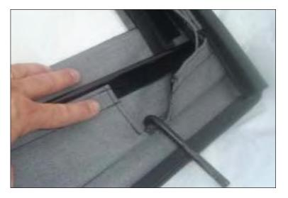
19. Reinstall upper doors. Insert pins into grommets in lower doors. Fasten snap at front of upper door. Slip plastic strip on bottom of door skin into retainer on lower door.
