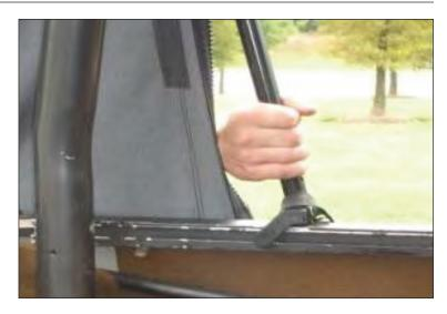
9. Pull down and insert rear corners of soft top into belt rail.
