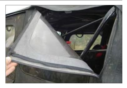
12. Slide plastic strip on front of side window into retainer channel on front support bow.
