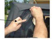
Start at the rear and roll the plastic along the bottom of the panel into the retainer on the vehicle. Then fasten the hook and loop strips along the rear of the panel to the top.
