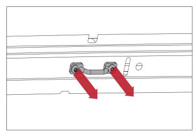
2. Reuse factory Torx Screws to install CB Mount with footman loop on outside as shown.
