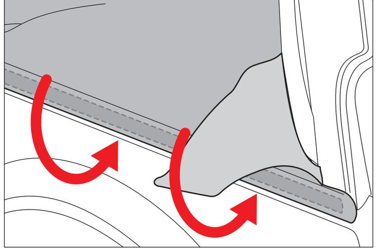
5. Roll plastic strip over edge and into rear groove of body tub. Repeat for opposite side.
