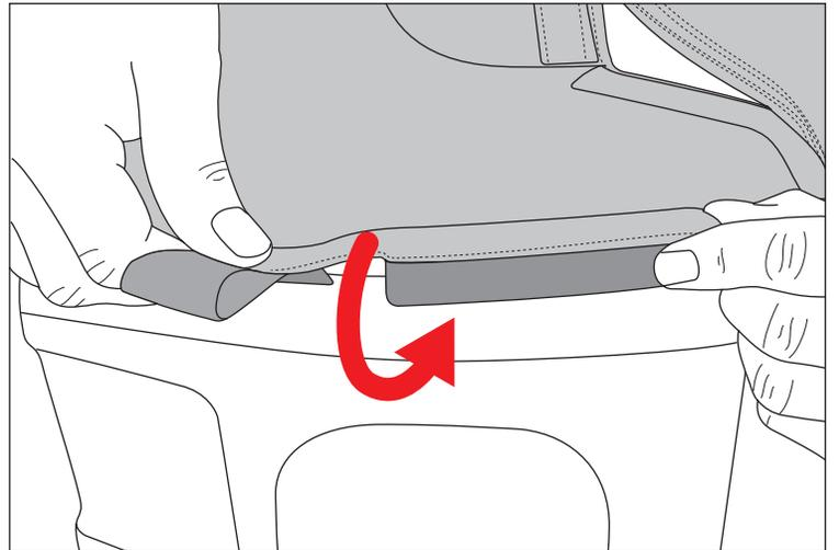
6. Wrap collars around rear sport bar and fasten hook and loop strips together. Repeat for opposite side.
