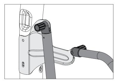
5. Once all bow knuckles are attached to mounting brackets, secure Quick Release Bow Knuckles to soft top bows with factory self tapping screws.
