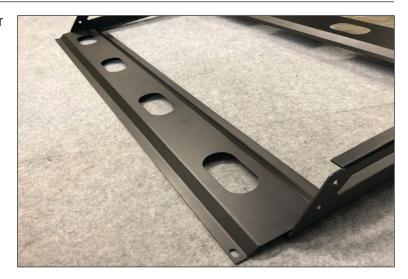
3. Slide the 5 center braces into place now attach with hardware. The first, middle and last center brace requires the longer button head bolt to pass through the center brace, rack and roof bracket. The second and forth center brace will use the shorter button head bolt to attach. Snug all the hardware but not fully tighten at this time. With it only snug it allows you to adjust the roof bracket when placing it on the Jeep later.
