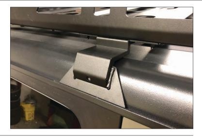
8. Now place the roof bracket outer clamp to the roof bracket. Attach with button head bolt and washer.
