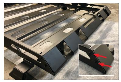
6. Now place rack on the Jeep roof. This must be done with two or more people. The rack weighs more than 100lbs so please use precaution before lifting. We also suggest place a blanket on the roof to avoid scratching the roof while placing the rack.
