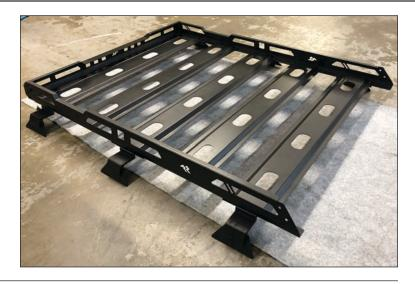
5. Now fit the front panel to the rack. It attaches with the short button head with washer and serrated flange nut. Now the rack is assembled fully tighten all the hardware except the hardware holding the roof brackets. These feet need to stay flexible to adjust to fit to the roof.
