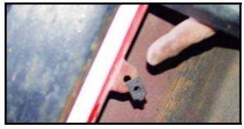
**Step 20:** Position armor onto lower side rocker panels. Make sure that it is evenly spaced before applying any pressure to armor. When satisfied with placement apply pressure to all areas to properly secure armor to vehicle. Secure bottom of rocker guards with hardware supplied.
