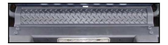
**Step 25:** Remove the (4) mounting bolts located on the front outer frame of the vehicle (2 per side). Remove the stock cover and replace with the new Frame guard. Reinstall with original bolts.
