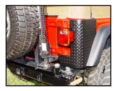
**Step 12:** Remove both left and right side rear tail light assembles. This will require the removal of 3 bolts for each light that are assessable from the inside of the tail light assembly and from the upper inside of the fender. The lower plastic fender cover can be pulled back without removing. The left side license plate holder and fuel filler neck will also be removed.
