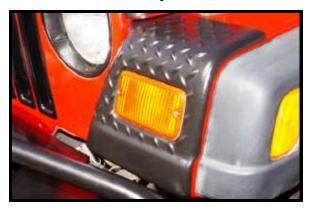
**Step 7:** Remove the hood stoppers and front turn signals from both front fenders.
