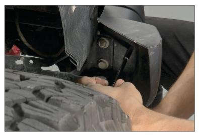
6. Now remove the inner splash shield brace. There are two bolts at the bumper and two bolts at the frame to remove.
