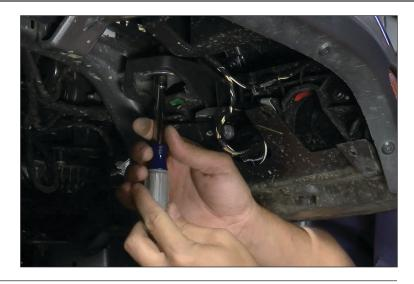
5. Pull splash shield down to reveal additional T25 torx screws to remove.
