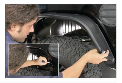
8. There is NO drilling necessary for this install. The nutserts will fit into the factory holes you marked in the previous step. To properly install we highly recommend using a nutsert tool. Insert nutserts into the Jeep body using the tool to crush the nutsert to the body. Take your time and assure each nutsert is crimped fully to avoid
