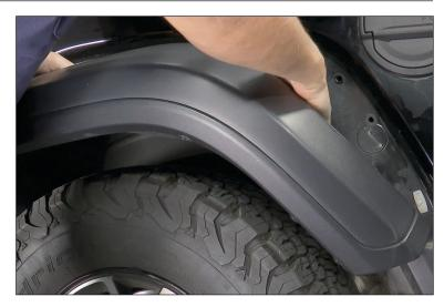
3. With the OE fender and liner removed clean the body of the Jeep in this area. This area retains mud and dust. If you see any scratches or paint is rubbed away, prep and paint areas to assist in rust prevention.
