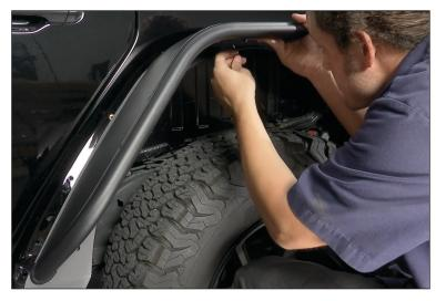
11. Now fully tighten hardware in a alternating pattern. Avoid using power or air tools. The last button head towards the rear of the fender is tight to the tube, it requires a short Allen head key to hold and tighten. This completes the install.
