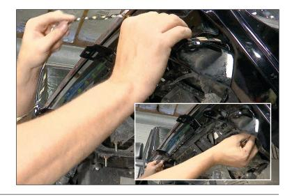
11. Now thread the LED lights to the fender and inside LED bracket. There is no need to overtighten the nut to the light. We strongly suggest appling a small amount of lock tight to the threads on the light then hand tighten. This will be sufficient enough to hold the light secure to the fender.
