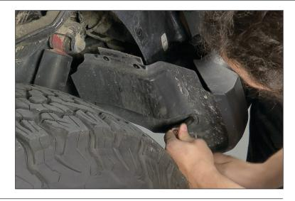
5. Remove the plastic shield from the bumper. It also has three M8 bolts attaching it.
