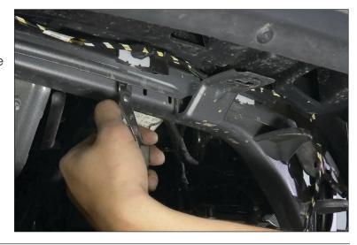
9. Remove the lighting hardness from the OE fender. Now cut the light socket/plug from the harness. We recommend staggering each cut so the wire splices don't stack on each other. Do Not cut the plug towards the rear of the fender to the main chassis hardness only cut at the turn signal.
