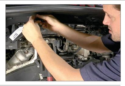
14. Next at the front of the fender attach the internal LED light bracket. Insert button head bolt through the OE fender bracket, steel fender bracket and LED light bracket, secure with washer and nut.
