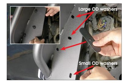
20. Now fully tighten all hardware. DO NOT use air or power tools to tighten. Tighten in a alternating pattern and repeat to fully secure. That completes the install of your front fenders.
