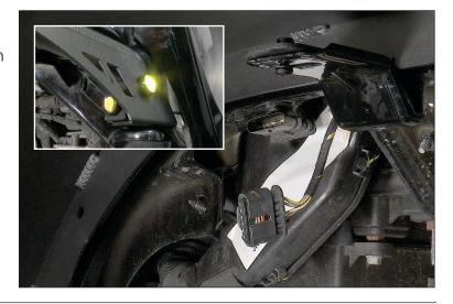
18. Now attach the remaining hardware of the fender to the Jeep body. Notice at the top mounting location requires a bolt plate because its to difficult to hold a nut between the fender liners. Hold bolt plate into position, see the bolt plate threads and thread the bolt to the nut plate.
