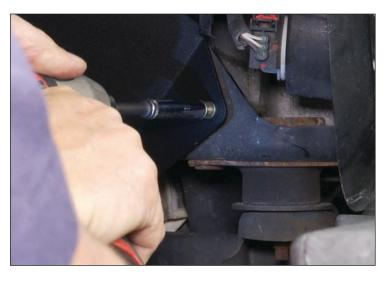
8. Now attached the rear self tapping screw to the Jeep body. That completes install.
