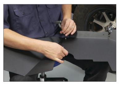
5. Use the OE hardware removed from step one to attach the inner fender to the Jeep. Place inner fender into position, thread the two bolts at the upper center of the panel, they thread up. Next thread the bolt near the front of the panel, it threads from the side. This bolt threads into a spring clip so make sure the clip is attached to the Jeep and is positioned correctly. At this time just hand tighten these three bolts.
