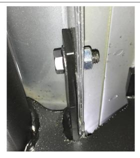
**Step 9.** Next, tighten the remaining hardware that attaches the bracket to the upper body mount.
