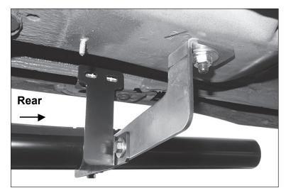
10. Temporarily remove Sidebar and Support Brackets. Use a 1/4" drill bit to drill 2 holes through pinch weld for each Support Bracket.
