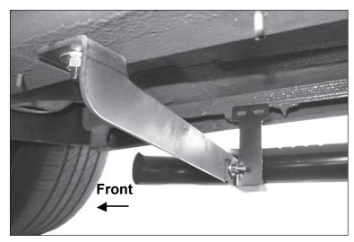
6. Move toward rear of vehicle and locate square plug in bottom of frame channel. Repeat steps 2-5 to install Passenger/Right Rear Bracket and Support Bracket.
