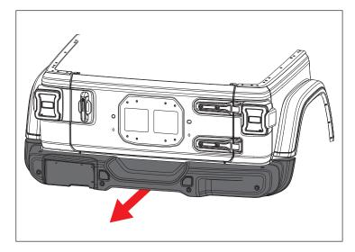
2. Remove the harness connctors from the sensors on the OE bumper. There is a gray clip on each one that can be pried backwards with a pick or screwdriver. Press the clip towards the wiring and pull the connector off.
