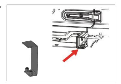
6. Affix Frame Mounting Brackets over the frame rails on both sides using M14 screws and washers underneath and sides.
