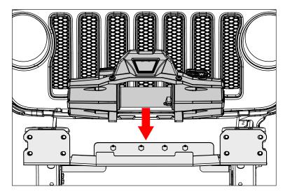
7. Remove factory winch delete plate and fairlead cover plate from Mopar Steel Bumper. Position Bumper on Frame Horn and Bottom Plate using Factory Tow Hook. Loosely attach with factory nuts. Tighten all Bolts. Attach lower air dam
