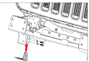
**Rugged Ridge Bumper**: Using supplied spacer, nut plate, and supplied 3/8" hardware, loosely attach Bottom Plate to lower cross member.
