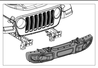
2. Remove OE Inner Frame Horn Bracket. Loosely attach Winch Plate reusing OE bolts.
