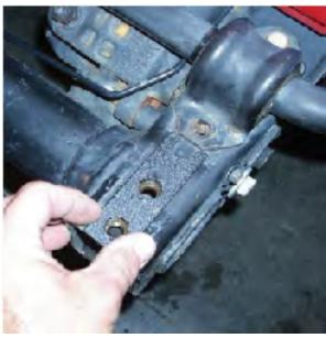
3. Mount winch to sub-frame making sure all lead wires have been connected. Two sets of mounting holes have been supplied for deferent winch designs. Most applications will use left mounting holes.
