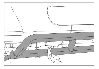
2. Attach the horizontal brackets to the body using supplied M8 bolts.
