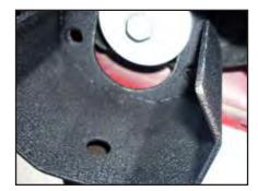
**Step 4.** Once all the nuts have been loosely threaded and the Armor is attached to the vehicle, begin tightening the nuts to 40-ft/lbs. Repeat for each mounting location.
