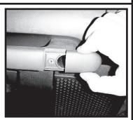
Step 2. Remove the hex head screws on both sides of the grab handle. Remove the handle.
