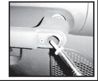
Step 3. Insert the supplied hex bolt thru the handle. Insert a spacer between the handle and the dash. Start the screw. Do not tighten. Repeat for opposite side. Once both screws have been started tighten both screws.
