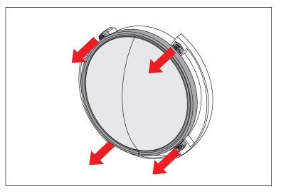
5. Install Pivitol Headlight Guard using factory screws in one of three configurations, vertical, horizontal, or diagonal. Each guard will work for both headlights.
