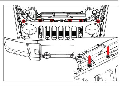
3. Pull bottom of grille away from vehicle to disengage metal clips on bottom rear of grille.
