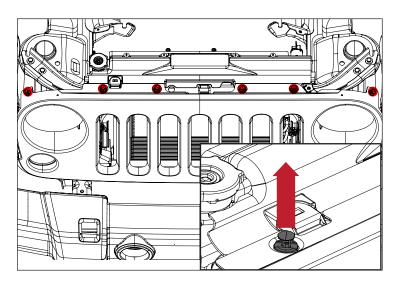
3. Pull bottom of grille away from vehicle to disengage metal clips on bottom rear of grille. Remove factory grille from vehicle.
