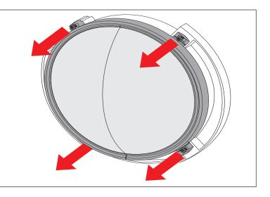
5. Using removed OE screws, install Elite Headlight Guard using T15 screwdriver or socket.
