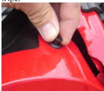
unscrew the plastic screws using a Phillips head screw driver.
