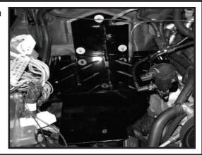
10. Check for clearance around the base of the Dual Battery Tray. Install both batteries onto tray and secure into position using supplied J-bolts and Battery strap. Slide EVAP solenoid over tab on Fuse Box Bracket. Reinstall air filter box to its original location.
