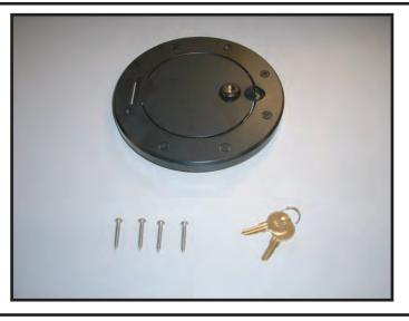
1. Install the Fuel hatch cover over the existing fuel filler trim. Make sure the door opens level.
