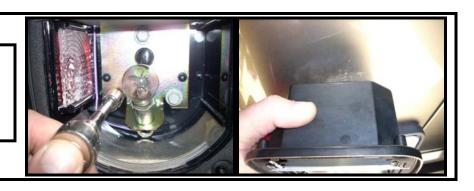
**Step 5:** Carefully pull the tail light wiring through the hole. Guide the connector through the hole.
