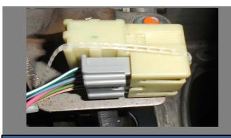
Locate the Brake Pedal Switch Assembly under the dash, in front of the Brake Pedal.
