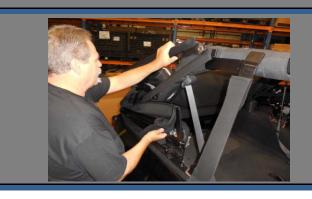
Line up the Motor Mounting Bracket with the Horizontal bottom bar Support Bar Assy.
