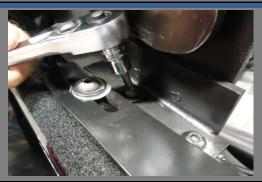
Tighten all the bolts using a 7/32" Allen Wrench.
