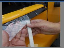
Remove the backing from the 27.5" Velcro Loop Strip, adhering the Velcro to the Jeep Tub under flange. Remove the backing very carefully to insure that the loop strip stays in the proper position: all the way under the flange.
