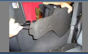
Fasten the Motor Cover using the  $1/4-20 \times 1/2$ " Screws and 1/4" thick washers.
