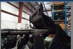
Operate the Frame Assy to the upright neutral position. "Neutral Position" means the forward section of the top assembly is just about vertical, and, with the power off, the top assembly does not drift open or closed.
