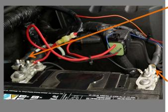
Connect the Red Positive (+) Wire with connector -interior (ref B.) to the positive (+) side of the battery wire accessory bolt, as shown in the photo.
