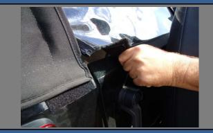
Partially unzip the rear window, on both sides, allowing access to the Velcro
