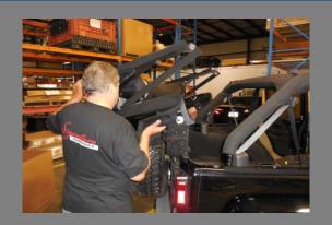
This is the 'heavy lifting" stage. The top assembly must be lifted over the spare tire, if you did not remove it. It is easier to do if the tail gate is slightly open, and the top assembly is maneuvered into position by moving one side up first about 5 inches, then the other side up by 5 inches, and so on. Move slowly and evenly. Slow and even movement will insure that body paint is not scratched, or that the roll bar covers are not nicked or torn, and fingers are not pinched.
