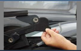
Cycle the Frame Assy down, allowing access to the mechanism for the attachment of the K-Plate Protection Pads.
