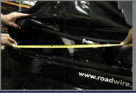
Measure from the center of the rear locator hole to the center of the screw head on the rear bow adjuster. The total distance should be 22.5".
