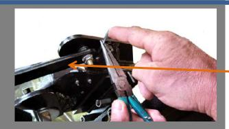
Carefully bend the limit switch levers to engage the Rear Trailing Arm when the top is in the open position.
