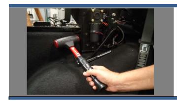
Using a dead blow hammer, tap the Motor Bracket into the correct position to achieve a 22.5" distance. Once alignment is achieved, tighten all 4 bolts. Repeat for the other side.
