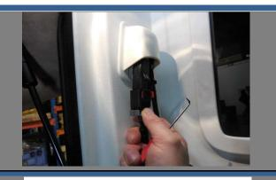
Use a pick to disengage the harness connector. Use caution to avoid damage to the connector.
