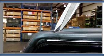
If you experience a water leak at the upper door it is recommended that you cut the seal as shown in the photo.
