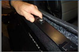
Attach the Horizontal bottom bar Support Bar Assy to the Side Plate Assy using two (2) 3/8-16 X 1" button head bolts and two (2) 3/8" thick washers. Hand tighten only at this time.
