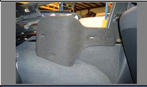
Align the Motor Cover with the holes in the Motor Plate Assy and the front hole in the Side Plate assy.
