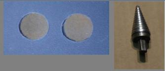
Using a step Drill, drill two 3/4" holes into the trim section, as marked. Using the switch, verify that the hole will accept the switch. Use caution when operating electrical hand tools.
