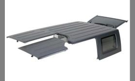
Once these are disconnected you can safely remove the Jeep's hard top. The top is heavy and awkward. Use two people to lift off. Use Caution when lifting heavy objects.
