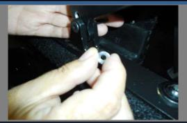
Attach the  $1/4 \times 20$ " lock nut to the FH bolt and tighten, leaving a 1/16" gap, between the lock nut and L-Arm; allowing the L-Arm to move freely and the FH bolt rotate freely.
