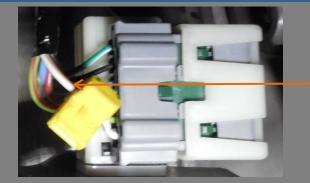
Locate the Wire Harness feeding into the Brake Pedal Switch Assembly. In the Wire Harness, locate the White/Brown Wire, which is closest to the bracket the Switch Assembly is attached to. Attach the T-Tap from the end of the Red/Yellow Wire of the MyTop Wire Harness to the White/Brown Wire.
