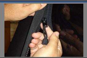
Insure that the rear window is at room temperature before installing. Move the top assembly to the close position to initially attach the rear window. Install the rear window, starting with the top zipper first. Note that the window edge with the sewn-in Velcro strip goes down, the zipper side is the upper side. The Velcro must face the inside of the vehicle.
