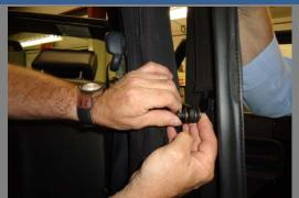
Fasten the Side Plate Assy to the Rollbar Bracket. Use one (1)- 3/8-16 X 1" Button Head Bolt and three (3) 3/8" thick washers (two behind the Rollbar Bracket and one under the Bolt Head).
