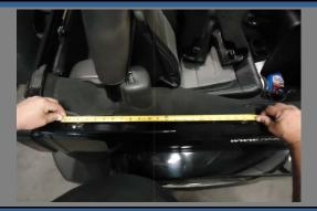
Measure 19 1/8" from the center of the rear locating hole to the rear edge of the Side Plate Assy.
