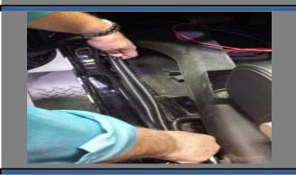
Remove the Drivers side floor sill plate cover, then route the Motor Harness Loom with Connector (LH/RH) (Wires # 7 & 8) along the underside of the floor sill plate cover, under the rear seat, towards the rear wheel well. Put the floor sill plate cover back on.
