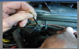
Zip tie the 40 Amp Sealed Fuse Receptacle (ref D.) to the plastic factory shroud.
