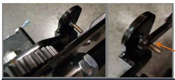
Place both trailing arms onto the studs.
