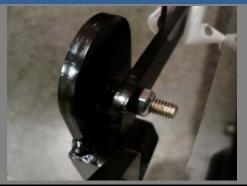
Install the 1/2" lock nuts, leaving a 1/16" gap between the nut and trailing arm.
