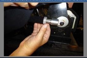
Operate the top to the open position. Pull the Rear Bow rearward. Mark your adjustment nuts, with a marking pen. Adjust each nut one full turn to gain proper fabric tension. Turning the nut Clockwise increases the tension of the fabric, removing excess fabric wrinkles. Turning the nut Counter-Clockwise decrease the tension in the fabric. Function the top and re-adjust as required.
