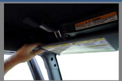
To open the top rotate both sun visors down and detach from the retaining clips.
