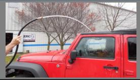
After completing the installation it is advised that you water test the myTOP using a garden hose. When spraying the top, angle your spray down at a 45° angle.
