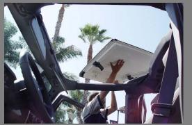
Carefully lift and remove the passenger side Freedom Top panel off your Jeep JK Wrangler and then store both panels in a safe place where they won't get scratched up.
