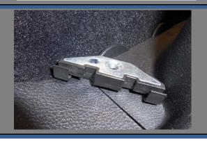
Once the top has been removed make sure the six (6) brackets, shown in the image, have been removed from the tub flange.
