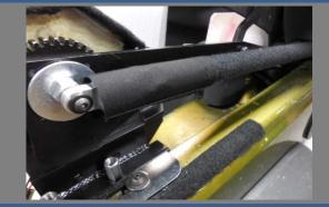
Proper placement of the the adjustment bolt fabric cover.
