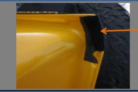
Attach the 43.5" section of Velcro Hook onto the upper section of the tailgate. Align on the upper edge of the tailgate continuing across and wrapping it around the tailgate section, as shown in the photo. Press firmly. Another set of hands may be helpful to insure that the Velcro attaches in a straight line.
