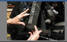
Depending on the fabric adjustment, you may need to increase the size of the slot in the fabric to achieve a proper fit. Use strong scissors or a knife. Use caution when working with sharp pointy objects.
