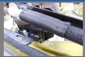
Rotate the seam to the underside.
