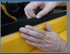
Once the loop is attached to the underside of the flange, carefully roll up the remaining portion of the loop up onto the the top of the Jeep tub.
