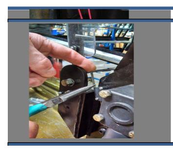
Bend the limit switch lever to engage the Trailing Arm when the top is closed.
