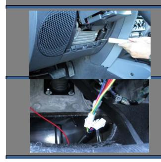
Notch out an area approx. 1" x 2" allowing for clearance for the switch assembly. Cut below the retaining clip. Use caution when using sharp pointy objects.
