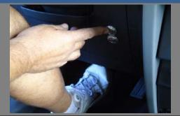
Press down on the brake pedal firmly. Push and hold the "TOP UP" button on the switch until the convertible top stops moving to the closed position.
