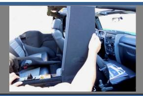
Position the Side Plate Assy onto the Jeep tub flange.
