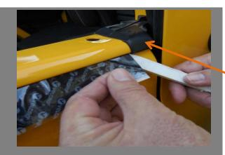
Attaching strips of Velcro in a straight line, and under the flange can be tricky. Proceed slowly to insure proper alignment and adhesion. Once the Velcro Loop is positioned under the flange, align the Velcro with the Factory Seal. Note that the "factory seal" refers to the rubber block located on the front portion of the Jeep tub rail where the rear door lines up with the tub when the rear door is closed. It is crucial to push the strip of loop fastener all the way up under the flange.
