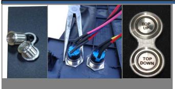
Carefully disconnect the Switches from the Harness assy, noting which wires attach to which pin; on the back side of the switch, then insert the switches through the switch bezel and the cut holes. Attach the retaining nuts to each switch. Make sure that both switches are properly aligned and tightened. Connect the switches to the wire harness, matching the wire colors.
