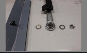
Place the 3/8-16 x 1.5" flat head bolt through the L-ARM and the black tinted Acrylic piece, then insert the Gold Washer followed by Interconnection Bar, the Silver Washer, and the 3/8" Lock Nut. Hand Tighten.
