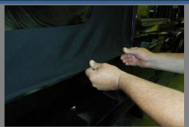
After attaching the top zipper, move top assembly down to aid in attaching the side zippers. Pull the fabric down and position the fabric. Relax any folds or bends in the rear window, and to insure snug fit, operate the top to the fully open position, then attach the rear window Velcro to the tail gate Velcro. Close the top to remove folds or bends in the rear window.
