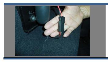
Make sure the connectors are firmly connected, as shown in the image. Pull gently to ensure the connectors are locked. When properly connected, you will hear a slight "click".
