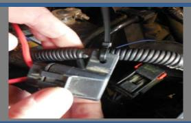
Secure the 12 Volt Sealed Relay (ref A.) to the plastic factory battery shroud using the provided zip ties.
