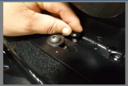
Align and attach the Jeep Top Assy Motor Plate to the tab of Horizontal Bottom Bar (HBB). Use a hole punch or screwdriver to aid in lining up the motor plate holes with the HBB holes. Once the four holes (two on each side) of the top assembly are aligned with the 4 holes in the HBB, you can hand thread the two (2) 3/8-16 x 3/4" bolts on each side to ensure proper alignment. Note: Do not use washers.
