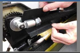
Once the rear bow is properly adjusted place the adjuster bolt fabric around the adjustment nut.
