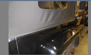
Fabric seated in the proper position. If the end of the fabric is not properly positioned, the end will flip up, the top will not fit properly.
