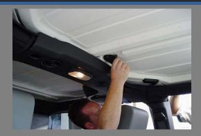
Starting from the driver side of your Jeep JK Wrangler, disengage the center latch closest to the windshield by rotating it counter clockwise. Then, disengage the latch in the center of the Freedom Top next to the sound bar as well as the one closest to the door pillar by rotating them clockwise.
