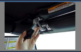
Grasp the padded handle and pull down, releasing the latch from the receiver. Repeat for the other side.
