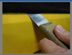
After you have checked that the loop section is in the correct position, use a tucking tool or fiber stick, firmly press the Velcro Loop into place.
