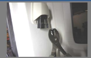
The rear window has a wiper on it like the windshield in the front. It also has a window washer, just like the front windshield. This window is attached to the Jeep's hard top, meaning there will be plugs that need to be un-plugged before you remove the top. The plugs are pretty tight, you may need to use a pair of pliers (LIGHTLY) to release them. There are pressure points on the sides of the plug that must be pressed to unplug them.
