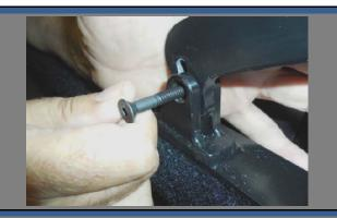
Remove the 3/8-16 x 1.75" flat head bolt.
