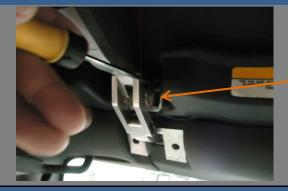
Loosen the Latch Assy Adjuster. Adjust by sliding the adjuster up or down to gain desired Latch Assy Tension.
