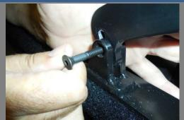
Align the slotted portion of the L-Arm (the short end) between the two tabs/brackets of the the Side Plate Assy. Slide the 1/4-20 x 1.75" FH bolt into the hole. Note: The FH bolt head should be installed from the outside of the assembly. Insuring that the beveled bolt head is on the outside of the Jeep, and the threaded end is on the inside of the Jeep tub.
