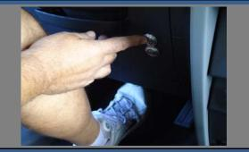
Press down on the brake pedal firmly. Push and hold the "TOP DOWN" button on the switch until the convertible top stops in the open position.
