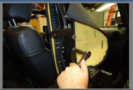
Attach the rollbar bracket using the M6 x 1.0 x 30mm hex head bolts. Leave the bolts loose.
