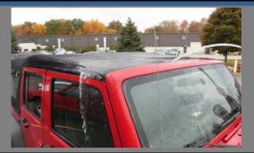
Spray the header area, making sure that no water leaks into the vehicle.
