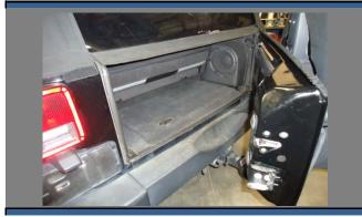
To close the tailgate, pull the rear window lower flap up while closing the tailgate.
