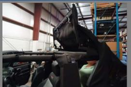
Operate the Top Assy to the neutral position using the "TOP UP" switch.
