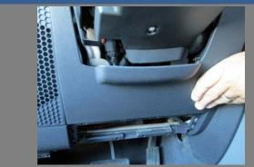
Carefully remove the lower trim access plate using a plastic fiber stick. Carefully remove the upper trim access plate, in the same way.
