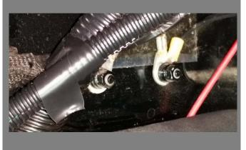
Fasten the Interior Ground Wire with Connector (Wire #4) to one of the two existing ground stud, where the clutch pedal would be located, slightly above the plastic "kick plate." as shown in the photo. Next, attach the two 12 volt motor relays, identified as (Wire #1) in the above diagram, to the factory bracket as shown in the photo. Use zip ties to secure the relays, but make sure the relays are attached high enough so that they are not kicked by the driver.
