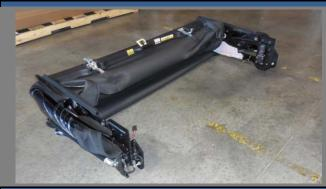
Remove the Jeep Top Assembly from the packaging. Place onto a clean surface.
