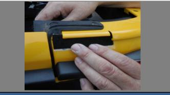
Place the Velcro Tailgate end sections: 3.5" onto the body flange. Align the Velcro piece with the inside edge of the opening.
