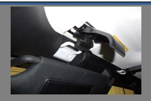
To remove your Jeep JK Wrangler's Freedom Top, flip down the sun visors and then unlatch the clamps securing it to the top of the windshield frame.
