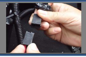
Securely connect the Motor Plug to the Wire Harness on both motors.
