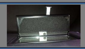
Attach the pre-cut, self adhesive, foam visor pad to the underside of the visor mirror. Insure that the pad and mirror cover are room temperature before adhesion. This pad will minimize the risk that a person may lose grip of the latch handle causing the latch handle to hit the mirror cover and break the mirror.
