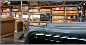
Photo shows the cut seal section, allowing for proper water drainage.
