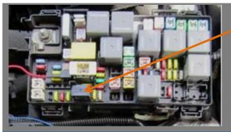
For the ignition feed connect the 15 Amp Fuse Tap (ref C.) into the open receptacle (M-14) inside the fuse box, as shown in the photo. To prevent the inserted wire from being pinched or cut, carefully notch the fuse box approx. 1/2" deep by 1/4" wide, using wire cutters. Use caution when working with sharp instrument to cut the notch.
