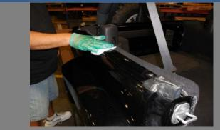
Clean the upper sheet metal surfaces, the sides, and under the flange of the Jeep tub with alcohol wipes in preparation for the Velcro sections. Note: Clean thoroughly to achieve proper adhesion. In addition, for proper adhesion we recommend both the Jeep tub and the Velcro be at room temperature for 1 hour before application.
