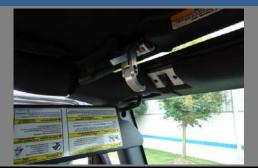
To close the top rotate both sun visors down and detach from the retaining clips. Rotate both sun visors outward against the door.
