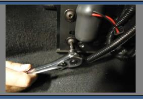
Loosen the three (3) pre-attached bolts on the Motor Plate Assy.
