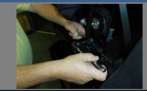
Use a 5/32" Allen wrench and a 7/16" open end wrench to tighten the lock nut to the FH bolt.
