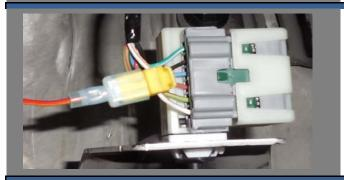
Insert the Male QD connector on the Red/Yellow Wire of the MyTop Wire Harness into this T-Tap.
