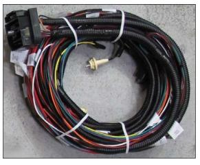
Locate the Engine/headlight harness; this will be the harness with a large rectangular bulkhead connector pre-installed. This harness will have connections for the headlights, horn, front turn signals and marker lights, as well as connections for components on the engine and for the start, charge, and ignition systems.
