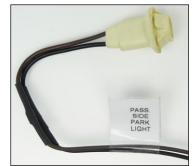
The park light requires two wires to work properly. A factory style socket comes pre-installed and will have a label reading "PASS. SIDE PARK LIGHT". The wires spliced to the brown and black wires of this molded connector are:
