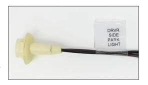
This connection will provide power and ground to the left/driver side park light. This is a two wire molded connector, these wires are:
