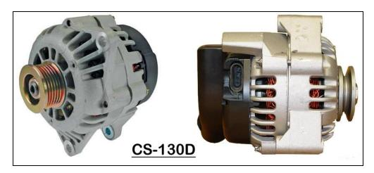
The GM CS-130D can be spotted by their lack of an external fan behind the pulley. These alternators have an internal fan. They also have a plastic casing on the back. These alternators have an elongated oval, four pin sealed connector, seen in the image above. The regulator will be marked P,L,I,S. This type of alternator was used on many engines, including the GM LS series, Vortec and Gen. III Vortec truck fuel injected engines.
