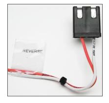
out the other side to the backup lights. When the shifter is put into the reverse position, contact is made between these two pins. This allows current to flow from one pin to another, transferring power through the switch out to the backup lamps.
