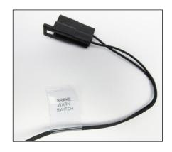
forward or back because of line pressure differences. This is usually caused by broken/leaking brake line or faulty caliper or wheel cylinder. Please be aware this is a pressure switch not a fluid level switch.
