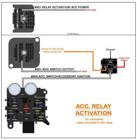
If you are installing a relay that will operate an electric fuel pump, water pump, fog lights or some other component that you want to activate with a toggle/rocker switch:
