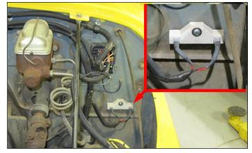
Route the Red/White #920 wire to its proper connection point, according to the diagrams mentioned on the previous page, and cut to length. Install the appropriate terminal for your connection, and
