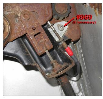
**Black**: 18 gauge wire, printed **#968 BRAKE WARNING SIGNAL**, this wire sends a ground source to the brake warning light in the dash, causing it to illuminate when the parking brake pedal is down. This wire can be seen in the <u>Gauge Cluster Schematic</u> on page 62.
