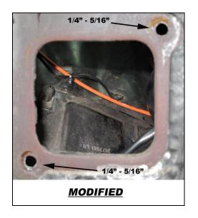
With the holes enlarged, the fuse block can now be mounted.
