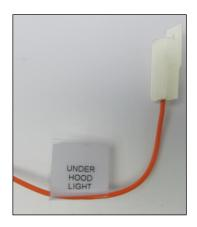
For the light to function it only requires a power wire. The light is turned off and on by a mercury switch inside of the light making contact when the hood/light is in the up position.
