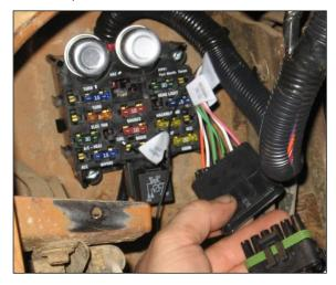
Once the tail harness has been plugged in it can be routed toward the rear of the Jeep, it will route exactly as the factory harness you removed routed. This routing will depend on the model of Jeep you have:
