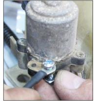
**Black**: 16 gauge wire printed with #969 HORN GROUND, this wire will provide the Horn with a ground source. This wire is part of the integrated ground circuit in this harness; it can be seen in the <u>Engine Ground Schematic</u> on page 13. This wire will be open ended and may not be needed on most applications.
