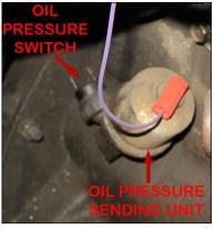
Locate the 18 gauge purple wire printed #922 OIL PRESSURE SENDING UNIT.
