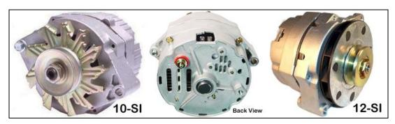
The GM 10-SI and 12-SI alternators are easy to identify. They will have an external fan behind the pulley, the 12-SI having enclosed style fan blades, and a two pin connection. This 2 pin connection can be seen on the middle image in the diagram above. These are also known as "Delco" or "Delcotron" alternators.
