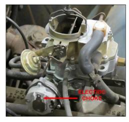
From the factory, the choke would only open when the engine had oil pressure, as in engine cranking or running conditions. This was done through the oil pressure switch, seen in the photo to the right and mounted in the picture at the top of the page. When the switch reads the appropriate amount of oil pressure, it closes or connects the two contacts.
