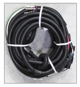
The final piece of the puzzle is the tail harness, this be the longest of the harnesses but has the fewest amount of wires and connections. This harness will provide power to the rear exterior lights and also send a signal from the fuel tank to the fuel gauge. This harness plugs into a connector found near the fuse block on the interior harness.
