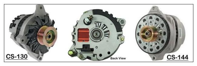
The GM CS-130, CS-121 and CS-144 alternators closely resemble the SI series alternators. They will have an external fan behind the pulley and they generally have some plastic casing on the side and back. These alternators have a four pin sealed connector, seen in the photo below and in the middle image above. The regulator will be marked P,L,S,F. This type of alternator was used on GM TPI and LT1 fuel injected engines among other late 1980's to mid 1990's GM vehicles.
