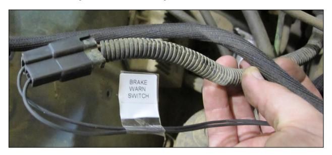
Those with a single pin brake warn switch; a pigtail to the one pin switch will be needed.
