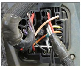
Connection of the engine bay harness will begin with the routing and connection of the exterior lights.
