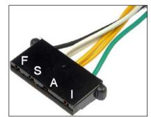
Terminals have been provided that will fit this connector, seen in the photo to the right. This will allow you to make a factory style connection.
