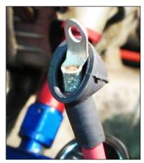
Be advised this heat shrink will have to be removed before the rubber boot can slide back down the wire if the charge wire is ever to be removed.
