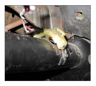
At this time the dash can be reinstalled over the column, but do not re-install the mounting bolts at this time.
