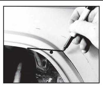
Step 11. Draw a horizontal line from the contour line inward towards the wheel well at the top of the third bolt hole. Repeat for opposite side.
