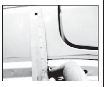
Step 32. At the bottom of the rear portion of the wheel well housing measure a distance of 1 5/8 inch from the the wheel well towards the rear of the vehicle.
