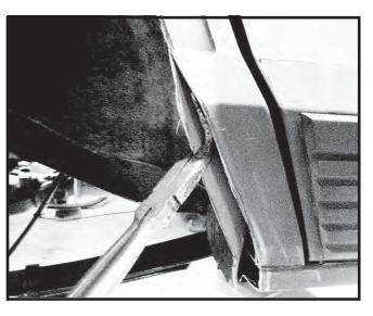
Step 38. Install the dog leg shaped trim piece on the door edge. At the rear door opening fit the trim against the body. Secure the trim in place with the supplied self tapping screws. Use the dimples in the plastic as guides for the screws. Do not overtighten. Repeat for opposite side.
