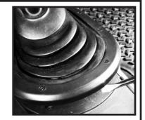
Step 3. With a screwdriver, seperate the lower ring from the boot joint.
