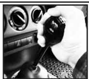
Step 2. Remove the existing bezel with a flat tool (e.g. Screwdriver). Pry up the rear side of the bezel releasing the two attached clips.
