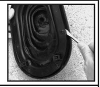
Step 4. Re-assemble parts using your Rugged Ridge bezel, joint boot and lower ring. Fasten parts together using the 8mm bolts and nuts provided.
